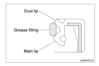
Fill the oil seal into the hole by using the oil seal guide and oil seal snap.
